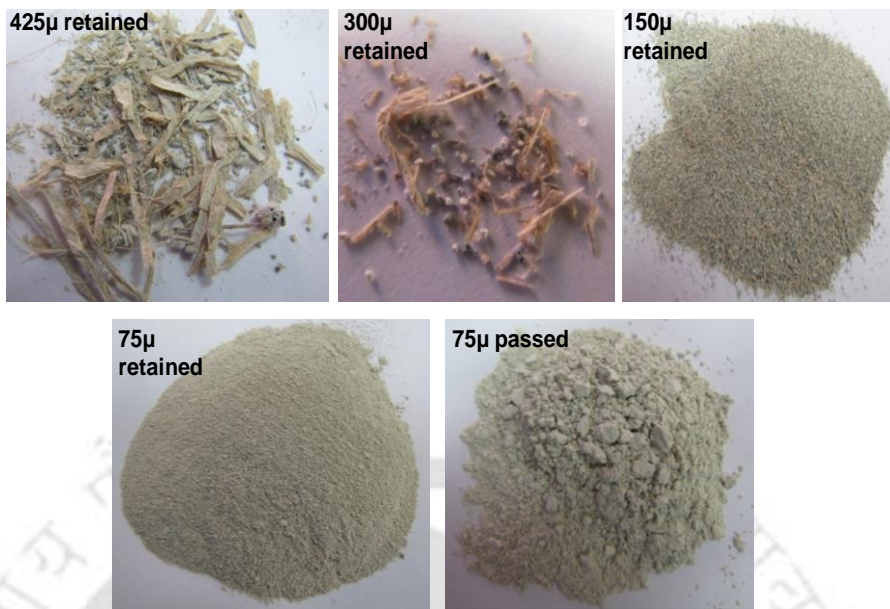
Fig 3.2a. Micrograph of heavy metals contaminated soil after passing various sieve
