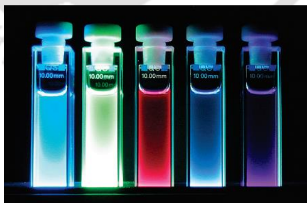
Figure 1.16 Observed emission from Ln(III) cations sensitized by 2-hydroxyisophthalamide (IAM) ligand irradiated with a standard laboratory UV lamp ( \lambda_{ex} = 365\text{ nm} ). From left to right, ligand only, Tb(III), Eu(III), Dy(III) and Sm(III) complexes. Reproduced with permission from ref. 178. Copyright 2009, American Chemical Society.
