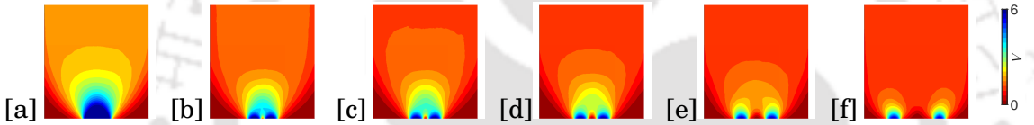
Figure 5.19: Spatial distribution of velocity V at different spacings L/d = a) 0.0, b) 2.5, c) 5, d) 10, e) 20 and f) 40 between the orifices, each of width W/d = 20 , placed on the silo base. The fraction of dumbbells for all the cases is X_{db} = 0.5 .
