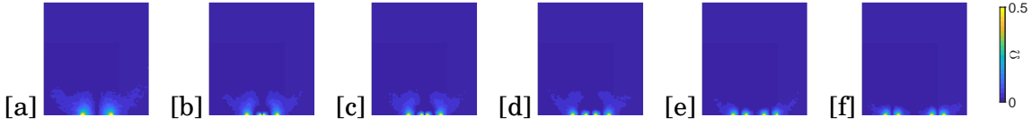
Figure 5.17: Spatial distribution of rotational velocity \Omega at different spacings L/d = a) 0.0, b) 2.5, c) 5, d) 10, e) 20 and f) 40 between the orifices, each of width W/d = 20 , placed on the silo base. The fraction of dumbbells for all the cases is X_{db} = 0.5 .
