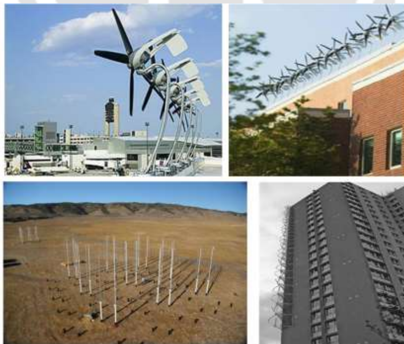
Fig. 6.1. Cluster/multirotor arrangement of small wind turbine
