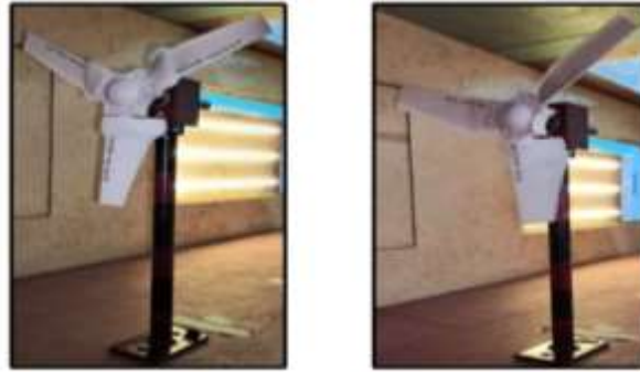
Fig. 4.18. Illustration of mixed airfoil SHAWT (a) MX1 (LS(1)042-E216), and (b) MX2 (E555-E387)
