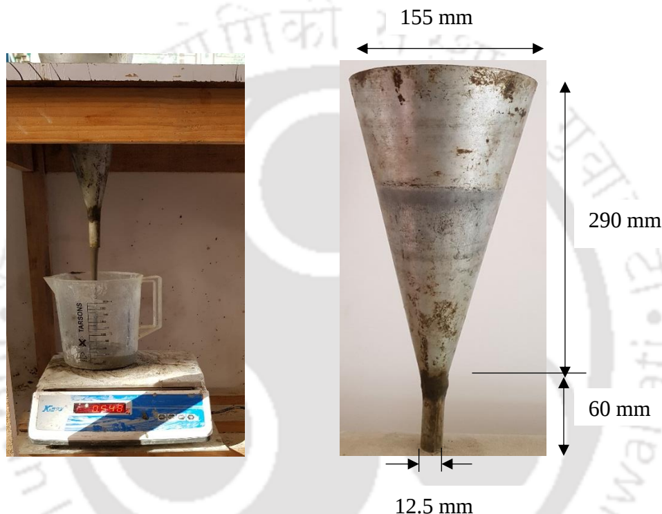
Fig. 5.4 Modified Marsh cone test
