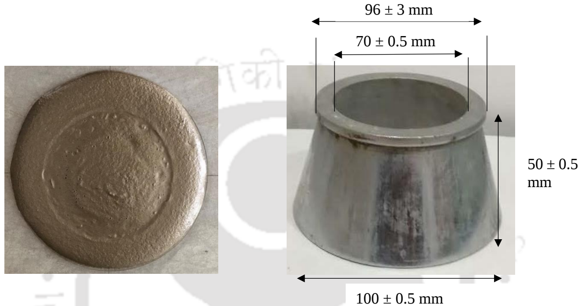
Fig. 5.2 Flow cone test
