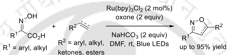
Scheme 1.43: Nitrile oxides generation by photoredox catalysis
