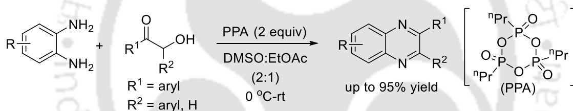
Scheme 2.4: Synthesis of quinoxalines from \alpha -hydroxy ketones
