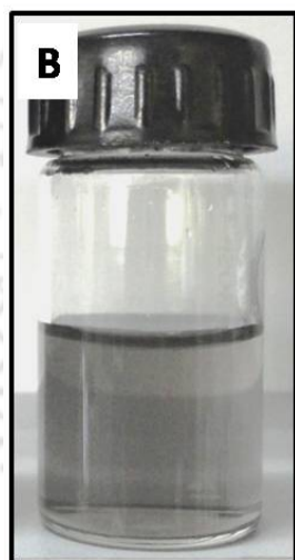
Figure 3.3.1.1 Scheme for MWCNTs-Enzyme conjugate synthesis using diimide activated amidation reaction. (A) Direct coupling reaction takes place using N-ethyl-N'-[3-(dimethylaminopropyl) carbodiimide hydrochloride (EDAC) and N-Hydroxysuccinimide (NHS) involving carboxylic acid group of oxidized MWCNTs and amine groups of respective enzyme, leading further to amide bond formation. (B) Image of aqueous dispersible MWCNT(SOD) biocatalytic conjugate, without any flocculation even after week of storage. (C) Linear absorption of synthesized MWCNT(SOD) biocatalytic conjugate at 500 nm as a function of its increasing concentration and also indicating highly homogenous aqueous dispersible nature respectively.
