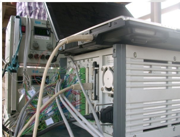
Fig. 5.2. Data acquisition system (MGCplus) along with notebook computer
