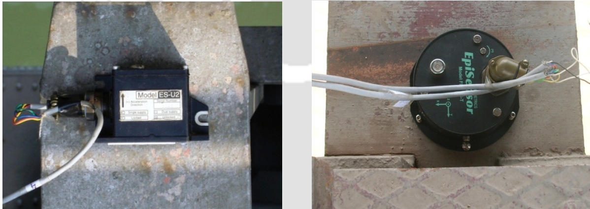
Fig. 5.1. Sensors for data acquisition: (a) EpiSensor ES-U2 and (b) EpiSensor ES-T
