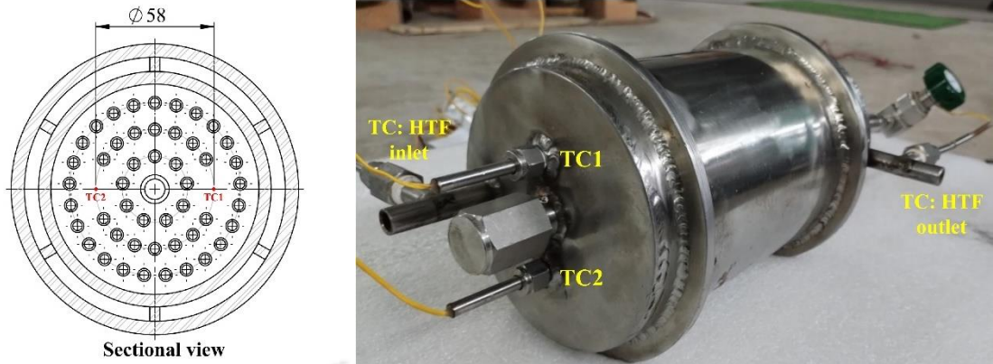
Fig. 5.2: (a) Radial location of the MH bed thermocouples and (b) photograph of the reactor.
