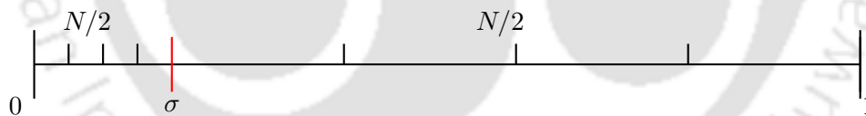
Figure 2.1: Shishkin mesh with N = 8 for left layer.
