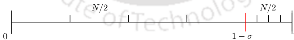
Figure 2.2: Shishkin mesh with N = 8 for right layer.
