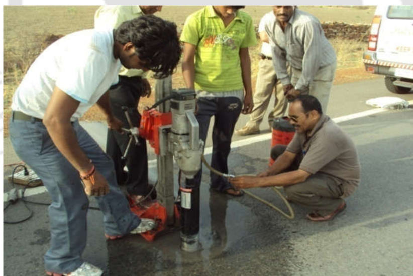
Photo 4.8 Full-depth core cutting of bituminous layers
