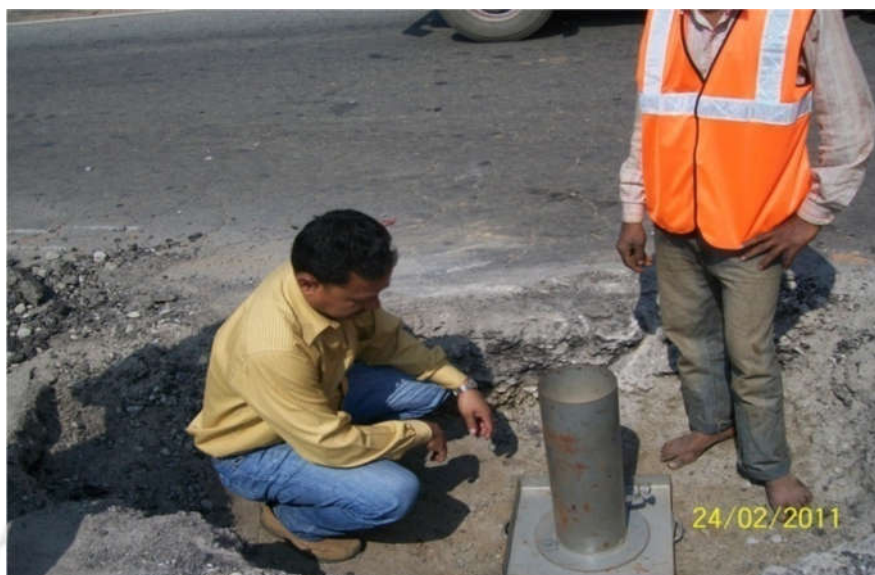
Photo 4.7 Field density test
