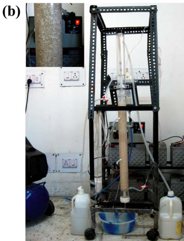
Figure 5.1.1. (a) Schematic representation of the re-circulated up-flow packed bed reactor (dimensions are not in scale). (b) Experimental set-up, (inset) Closer view of the reactor bed.
