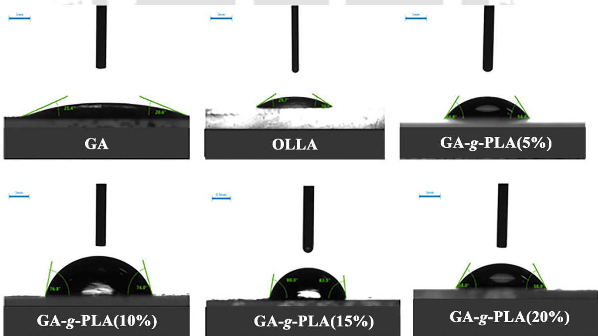
Figure 4.9. Contact angle analysis of GA, OLLA and GA-g-PLA bionanocomposites.
