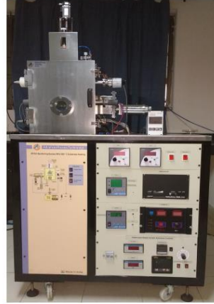
Figure 2.6: RF reactive magnetron sputtering system.
