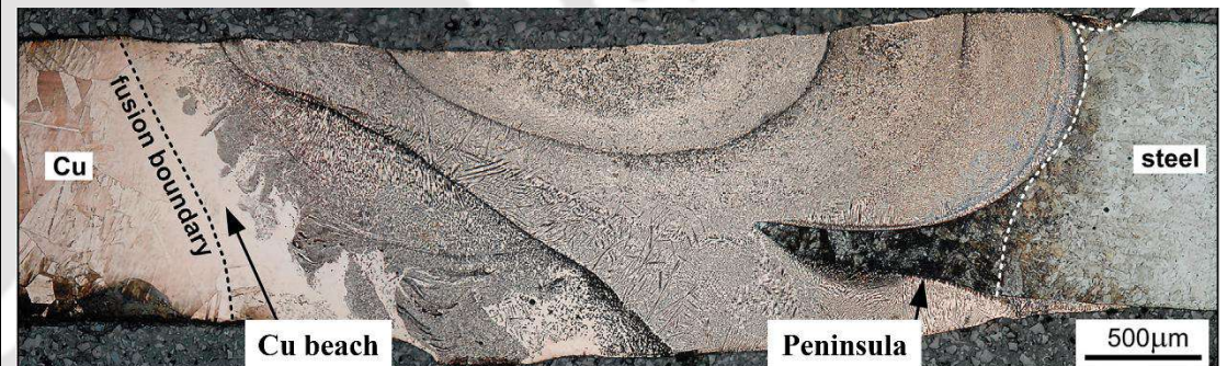
Fig. 2.13 Illustrates microstructural features (beach, peninsula, fusion boundary) of Cu-SS dissimilar joint (Soysal et al., 2016).
