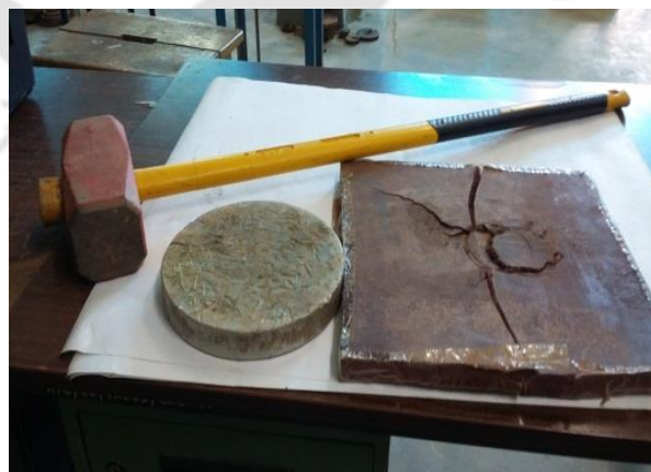
Fig. 3.5: Striker plates of different compositions – Cast steel and Rubber
