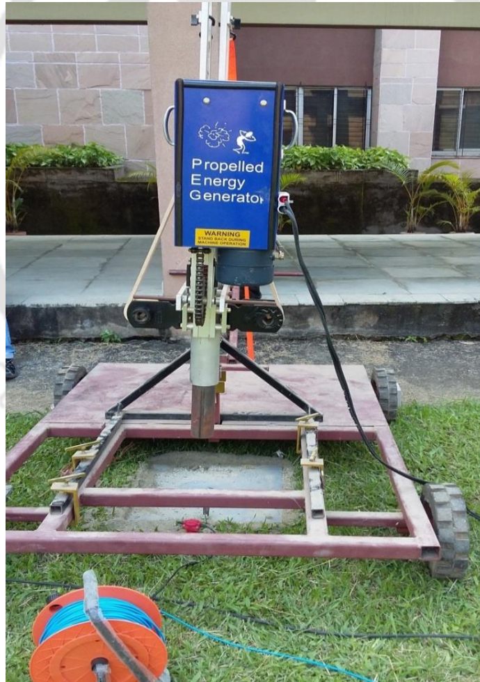
Fig. 3.2: A 40 kg Propelled Energy Generator (PEG) acts as an accelerated weight drop
