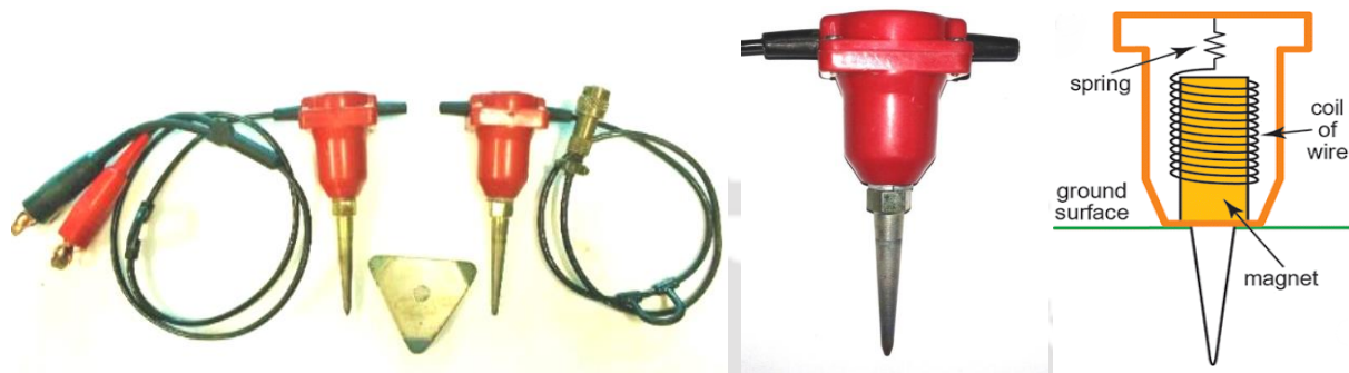
Fig. 3.3: (a) Geophones and their working principle
