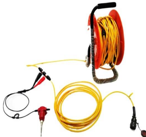
Fig. 3.8: (b) Typical layout of linear array of geophones for active MASW survey (c) Connecting mechanism of the geophones with the connector cable
