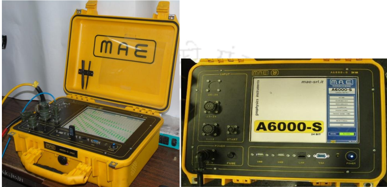
Fig. 3.4: 24-bit MAE Data Acquisition System (DAQ) used in the present investigations
