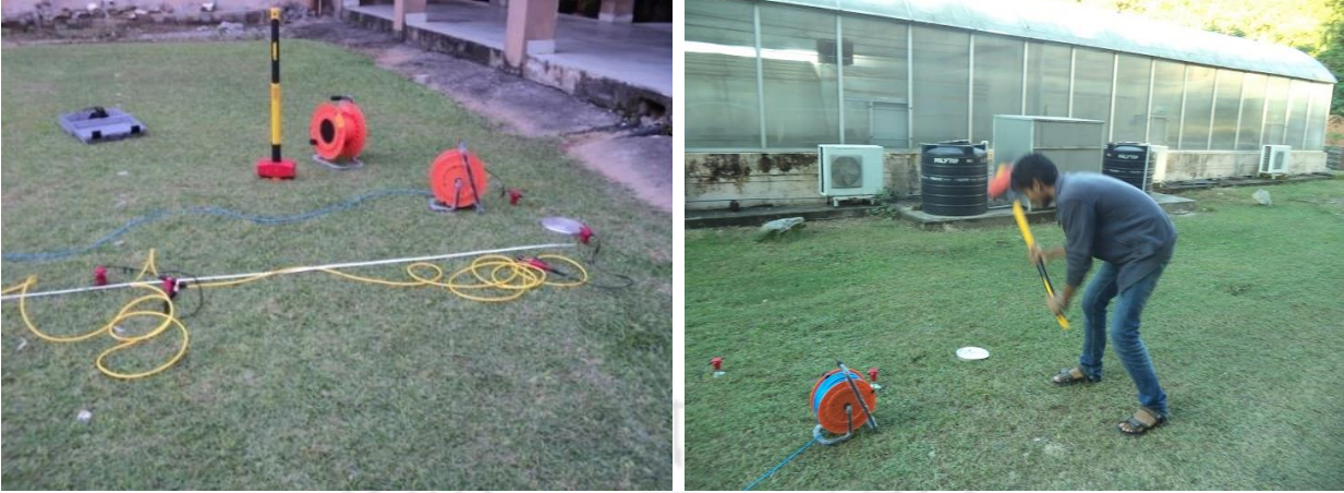
Fig. 3.1: A 10 kg sledgehammer operated by single personnel to strike the base plate
