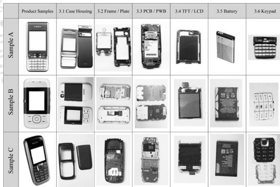
Figure 1.3: Dissected mobile phones of different price ranges
