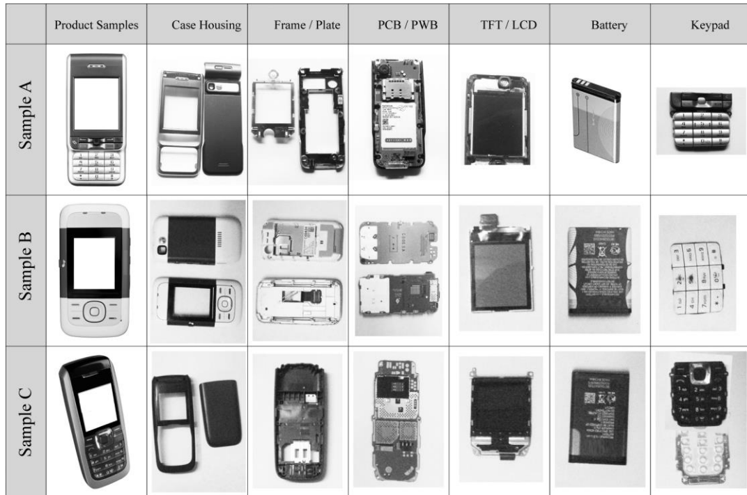
Figure 7-2: Product sample study of a mobile phone (Major modules of sample A, B and C)
