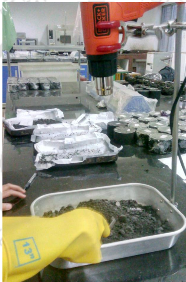
Figure 3.12 Loose mixture drying process
