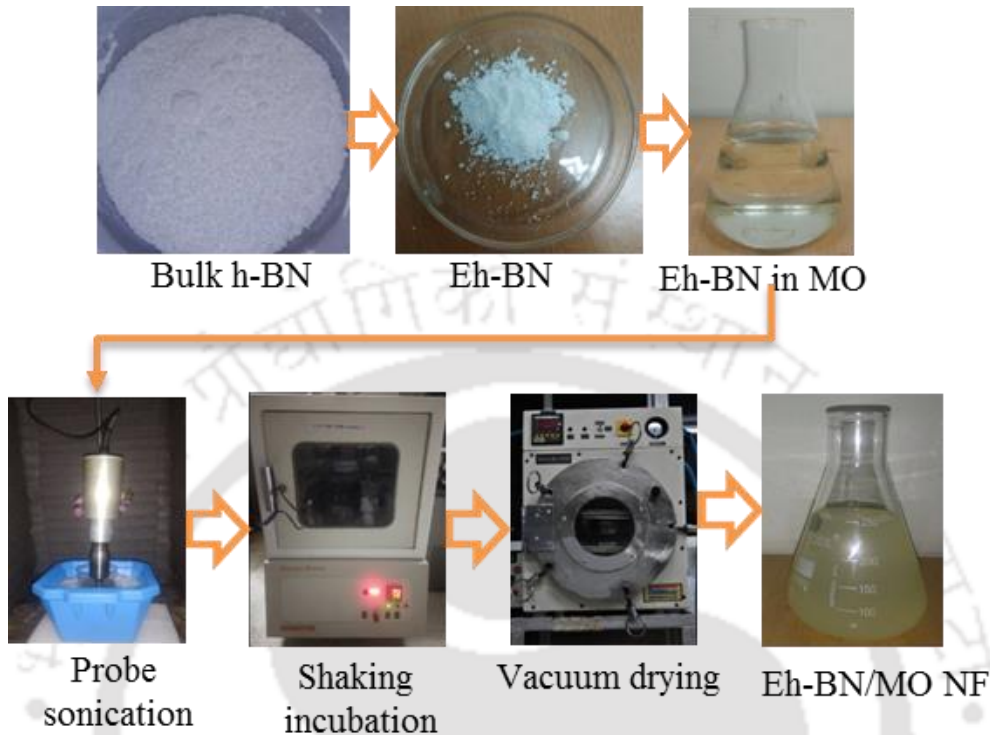
Figure. 2.5: preparation of NF as per two step method.
