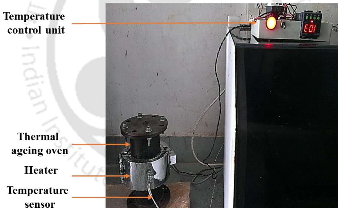
Figure 5.3: Fabricated setup of natural convection imposed accelerated thermal ageing simulator.
