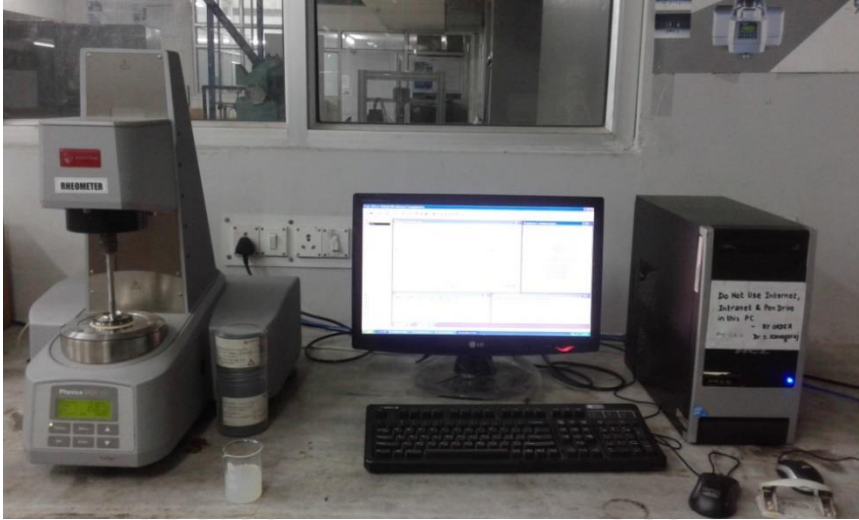
Figure 2.8: Rheometer to analyse the rheological parameters.
