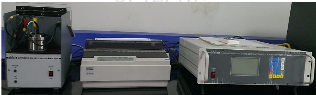
Figure 2.22: Tan Delta-DTR-3K Measuring setup (RTL, CPRI, Guwahati).
