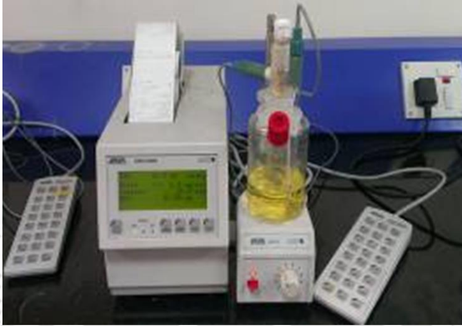
Figure. 2.7: Karl Fischer Titration method for moisture analysis.
