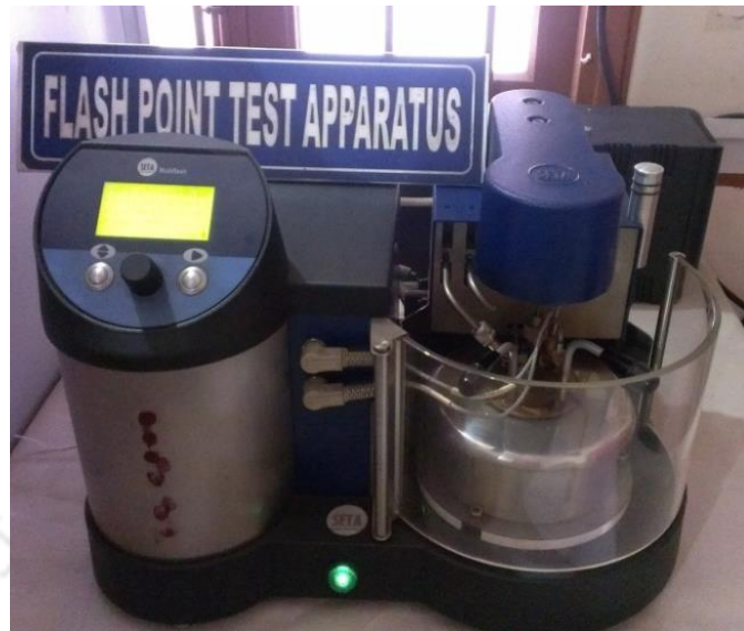
Figure 2.14: Pensky-Martens cup apparatus for flash point, (RTL, CPRI, Guwahati).
