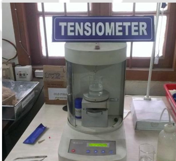
Figure 2.16: Tensiometer for IFT (RTL, CPRI, Guwahati).
