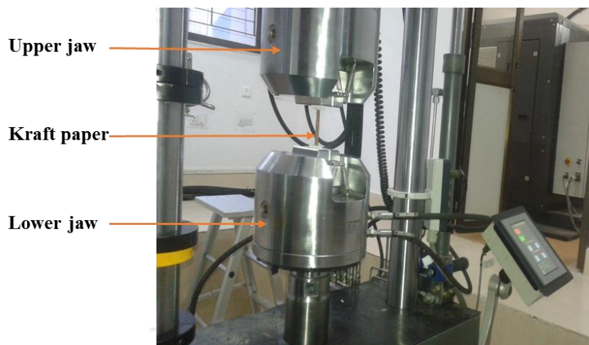
Figure 5.9: UTM used to measure the tensile strength of aged kraft paper.
