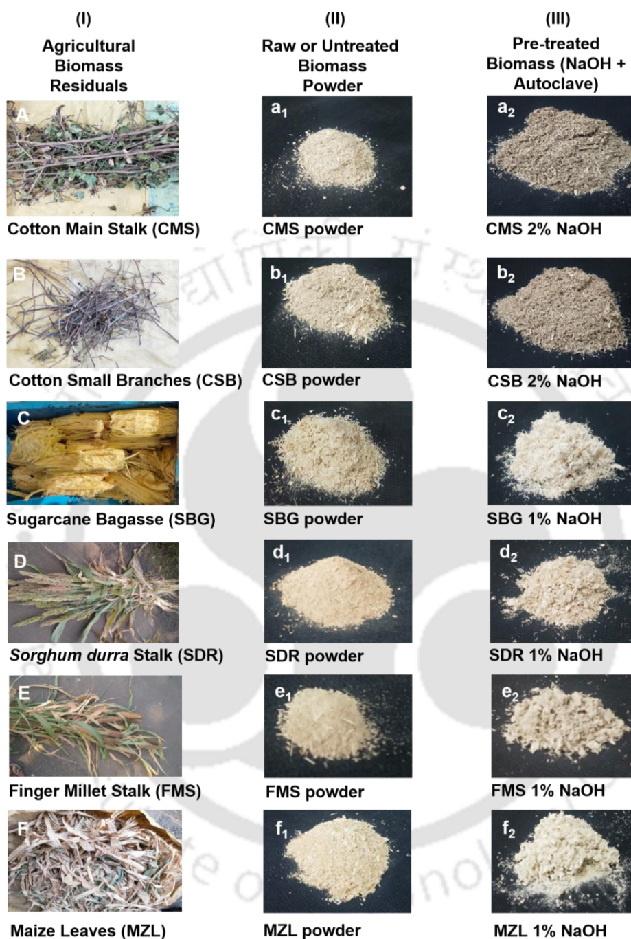
Fig. 5.1 Harvested agricultural residues biomasses (I-A-F), processed raw biomasses (II-a 1 -f 1 ) and alkali pre-treated biomasses (III-a 2 -f 2 ). A-a 1 -a 2 : Cotton (CMS), B-b 1 -b 2 : Cotton (CSB), C-c 1 -c 2 : Sugarcane bagasse (SBG), D-d 1 -d 2 : Sorghum (SDR), E-e 1 -e 2 : Finger millet (FMS) and F-f 1 -f 2 : Maize leaves (MZL). Alkali pre-treatment of these lignocellulosic biomasses was carried out using 1%, w/v NaOH for SBG, SDR, FMS, MZL and 2%, w/v NaOH for CMS and CSB, followed by autoclaving at 121°C for 20 min.
