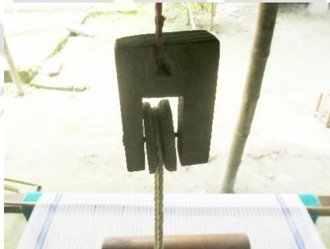
Fig 3.9(b). Gorai, (pulley)Used to connect the tension through treadle. ( Source:private collection, Besargaon. Photo:Self.Date: December 2023).
