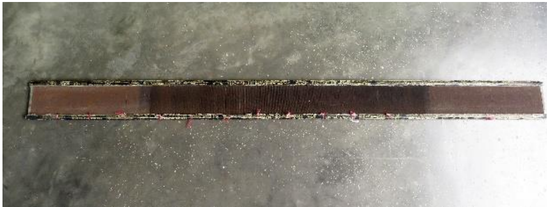
Fig 3.9(f) Rasw (Bamboo Reed used to dents the treads). Source: private collection, Besorgaon. Photo:Self.Date: December 2023)
