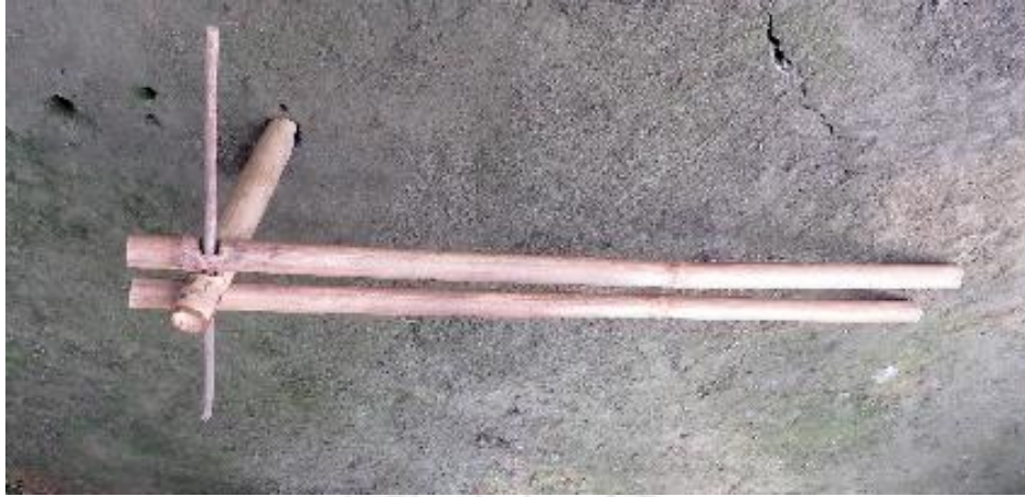
Fig 3.9(c) Gorkha (Bamboo Treadle) used to cycling during weaving. ( Source: private collection, besargaon. Photo:Self.Date: December 2023)
