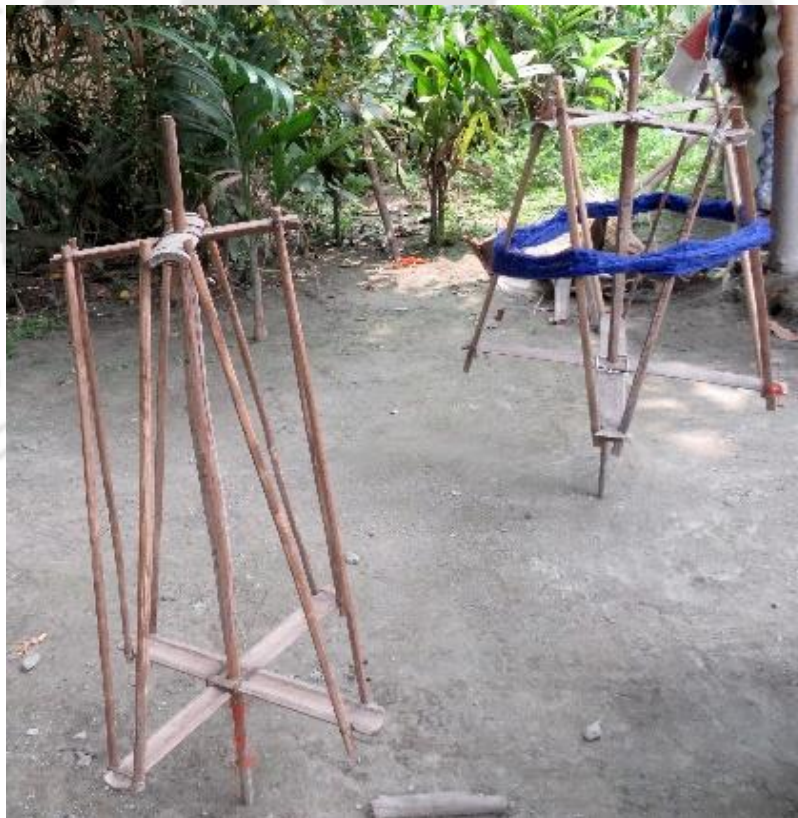
Fig 3.9(l) Swrkhi( Bamboo Swift, a weaving contrivance. ( Source: private collection, Besorgaon, Chirang. Photo:Self.Date:December 2023)
