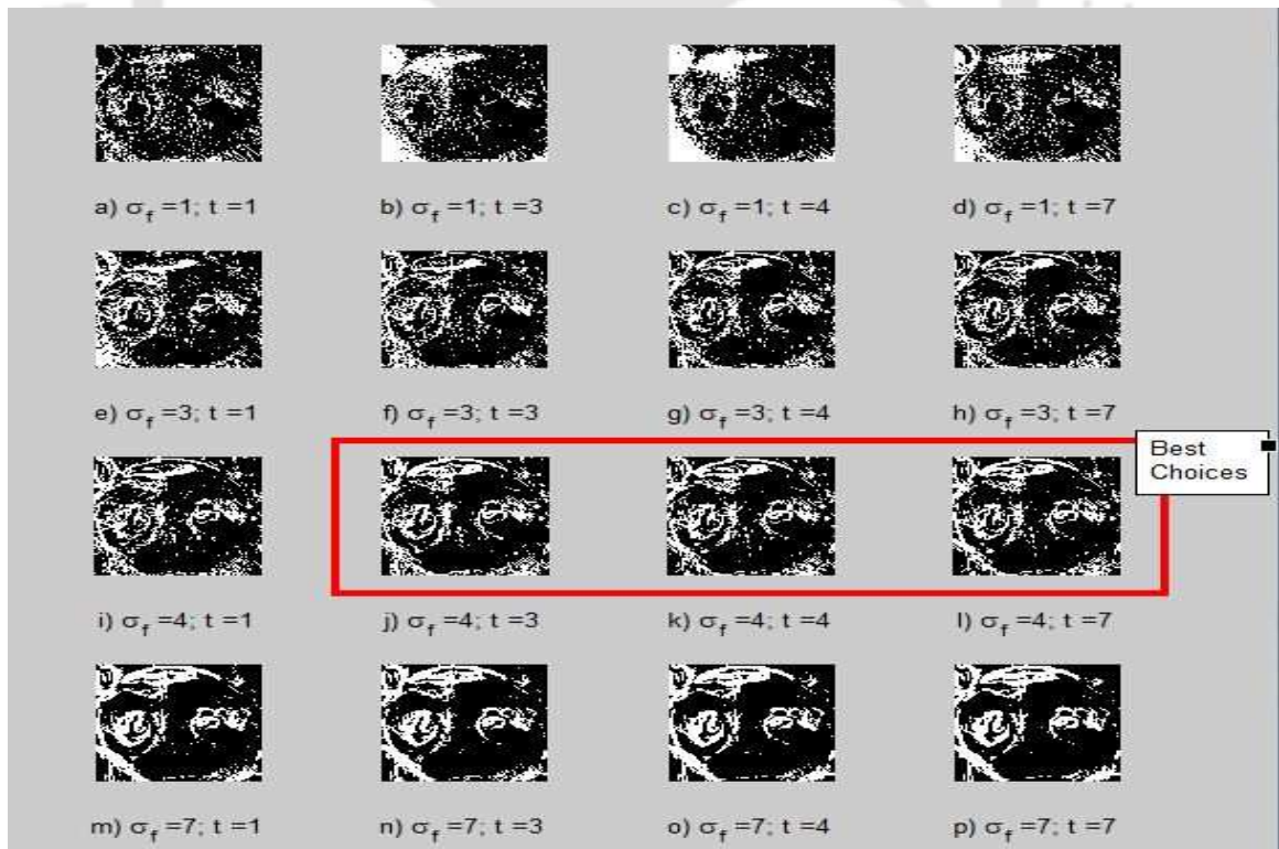
Figure 2.13: Impact of DGau pre-filtering and texture quantization on the muzzle of a Ghungroo pig (Fig. 2.12).
