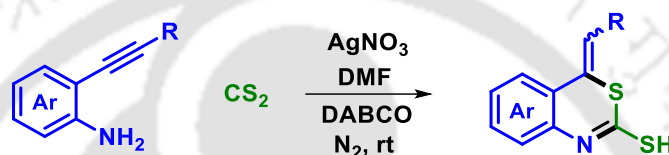
Scheme IB.3.3.1. Synthesis of 2-mercapto-4-benzylidene-4H-benzo[ d ][1,3]thiazines.
