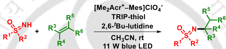
Scheme IA.2.1.4.6. Photocatalytic N -Alkylation of NH-sulfoximines via anti-Markovnikov hydroamination of alkene.
