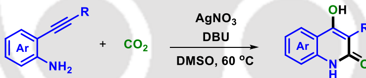
Scheme IB.3.1.2. Synthesis of 4-hydroxyquinolin-2(1H)-one.
