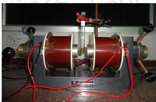
Figure 6.1. Photograph showing \text{Fe}_3\text{O}_4 NP dispersion (in \text{CHCl}_3 ) suspended between the poles of an electromagnet.
