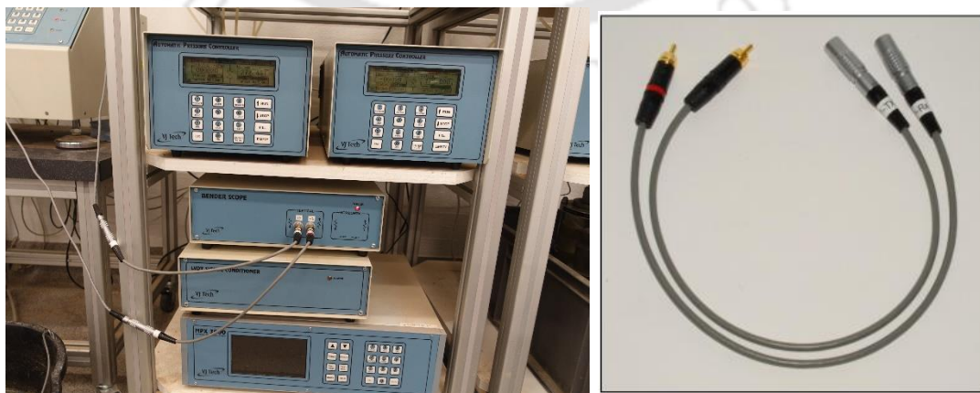
Fig. 3.15 Bender element scope system and leads for generation of input signals and monitoring the output signals
