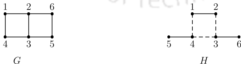
Figure 1.1: A graph G with three perfect matchings and a graph H with a unique perfect matching.
