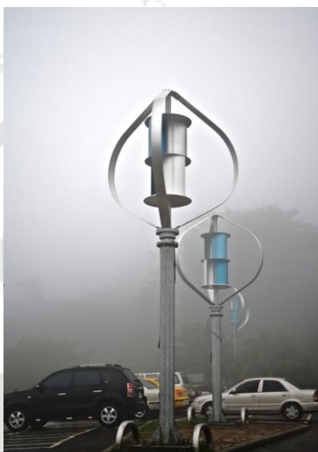
Figure 1.4: Historic Gold Mine Savonius–Darrieus combined VAWT in Taiwan (November, 2009). Source: Courtesy of Fred Hsu, reproduced under GNU Free Documentation License 1.2.
