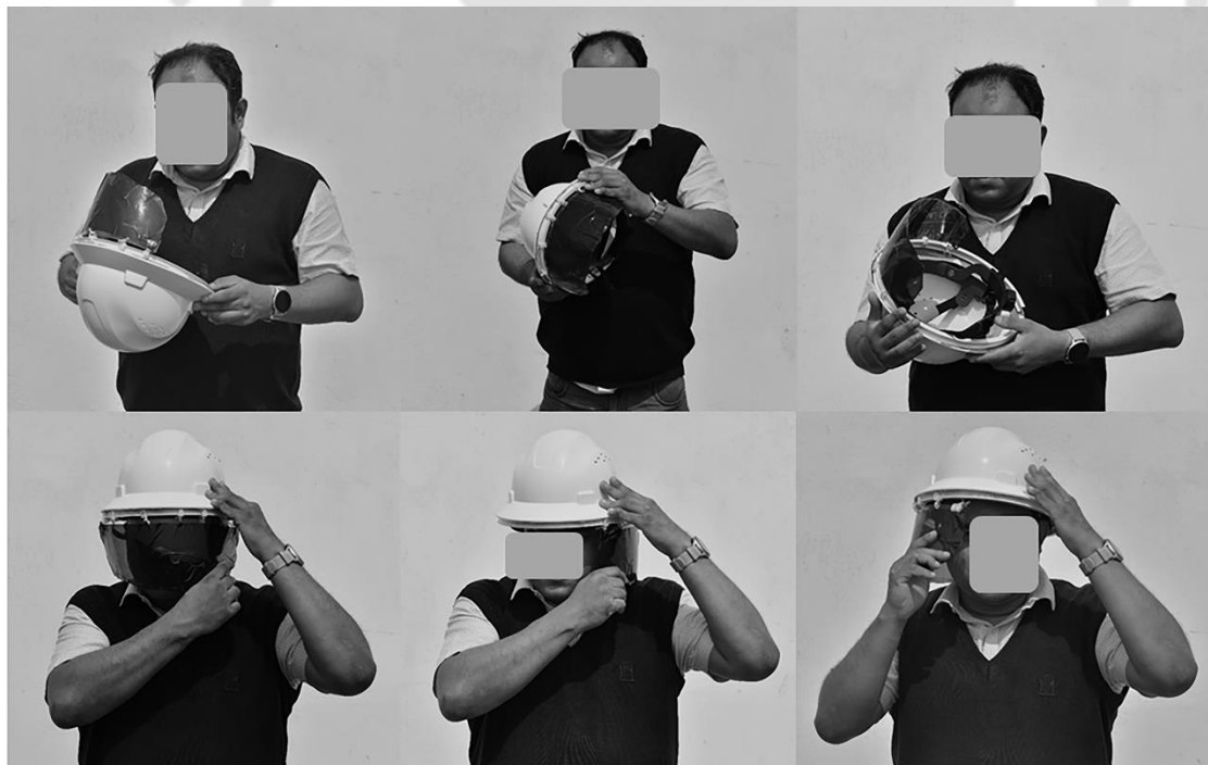
Figure 6.28. Usability testing of the anti-glare and anti-UVR eye protector (image: author)
