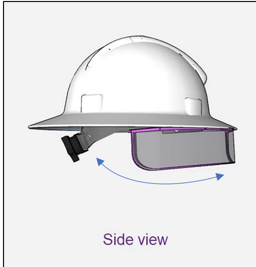
Figure 6.18. Mechanism of use of eye protector
