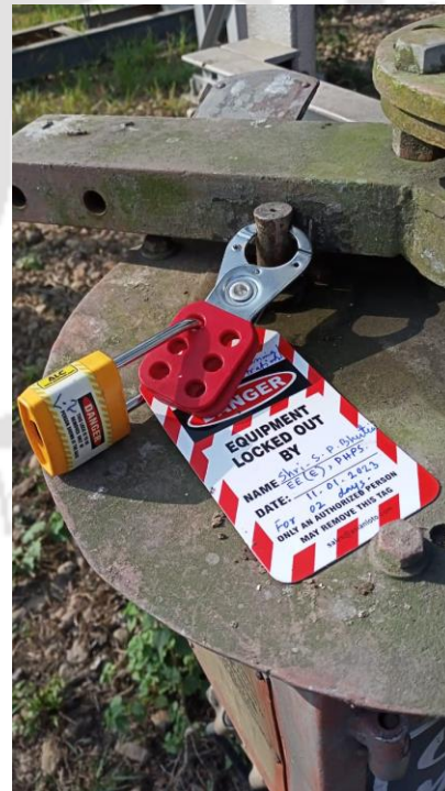
Figure 6.7. Photographs showing Lock Out Tag Out (LOTO) for electrical safety (image: author)
