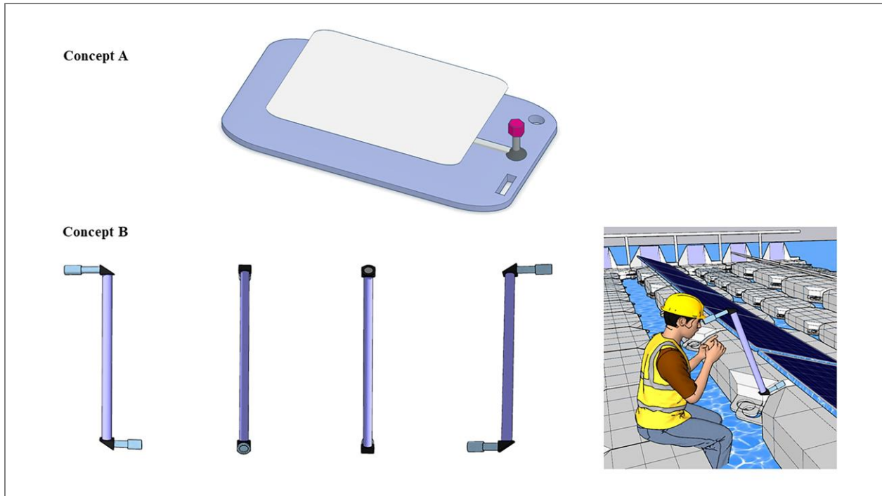
Figure 6.43. Concepts developed for maintenance mirror (image: author)
