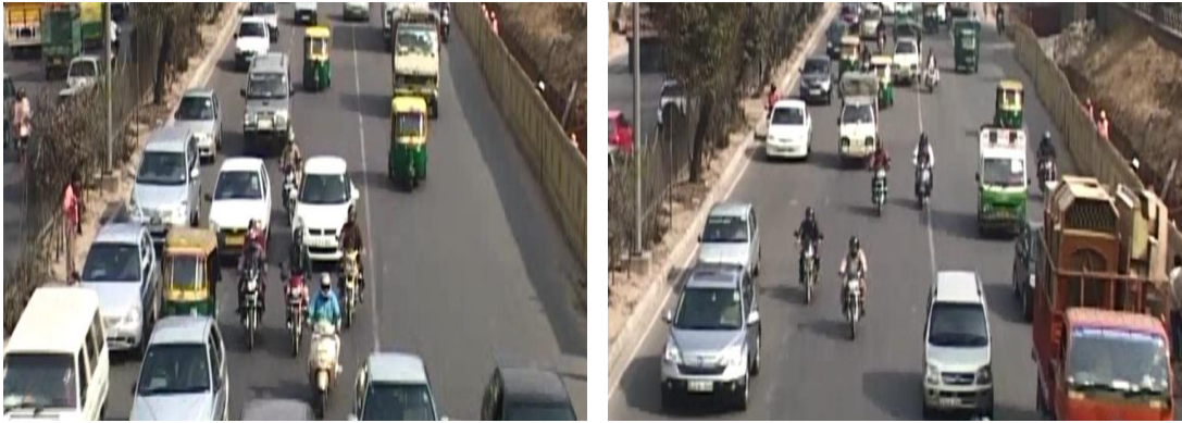
Fig. 4.1 Variable lateral gap maintained by MTW at two different scenarios
