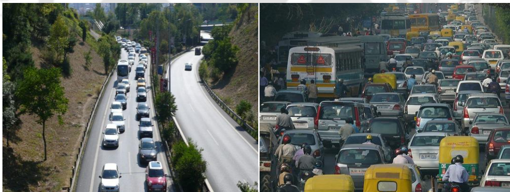
Fig. 1.1 Comparison of traffic streams with lane discipline (left photograph); without lane discipline (right photograph)
