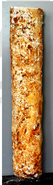
Fig.3.41: Pre-test shape of a typical stone column ( L/d_{sc} = 5 , S/d_{sc} = 2.5 )
