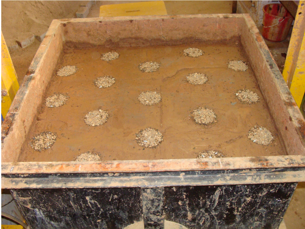
Fig.3.40: Stone columns in a typical test bed
