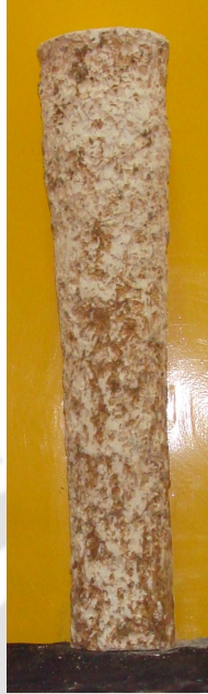
Fig.6.35: Post-test deformed shape of a typical central stone column in composite foundation bed ( L/d_{sc} = 5 , h/D = 1.1 , S/d_{sc} = 2.5 ) – Test series 11
