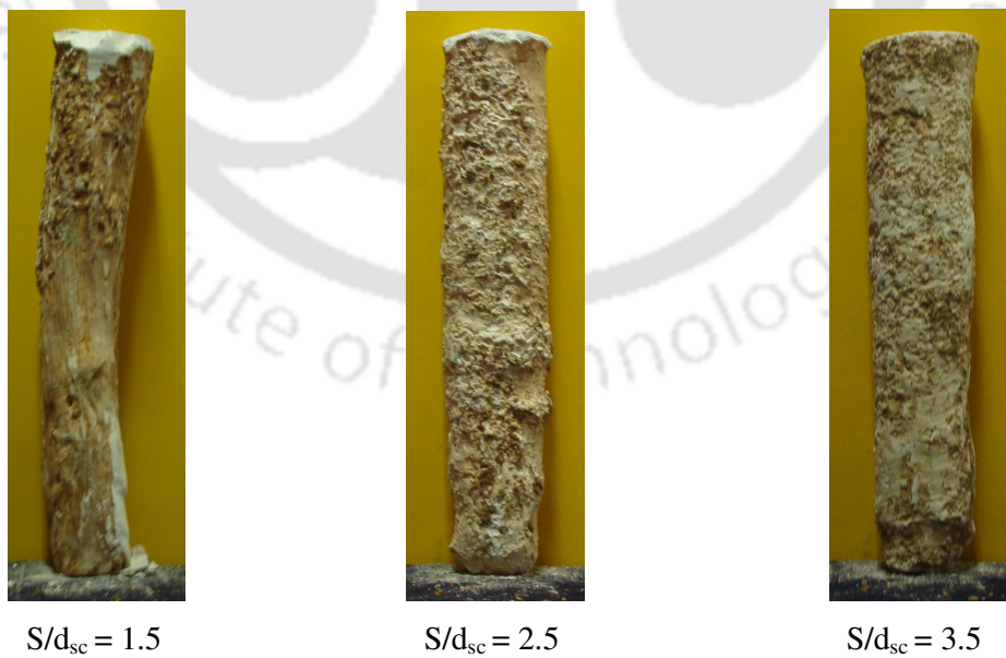
4.24: Post-test deformed shape of typical peripheral stone columns (L/d_{sc} = 5) – Test series 3
