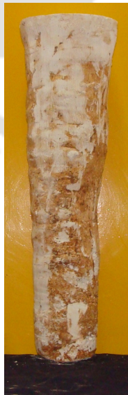
Fig.6.15: Post-test deformed shape of a typical central stone column in composite foundation bed ( L/d_{sc} = 5 , h/D = 0.53 , S/d_{sc} = 2.5 ) – Test series 9
