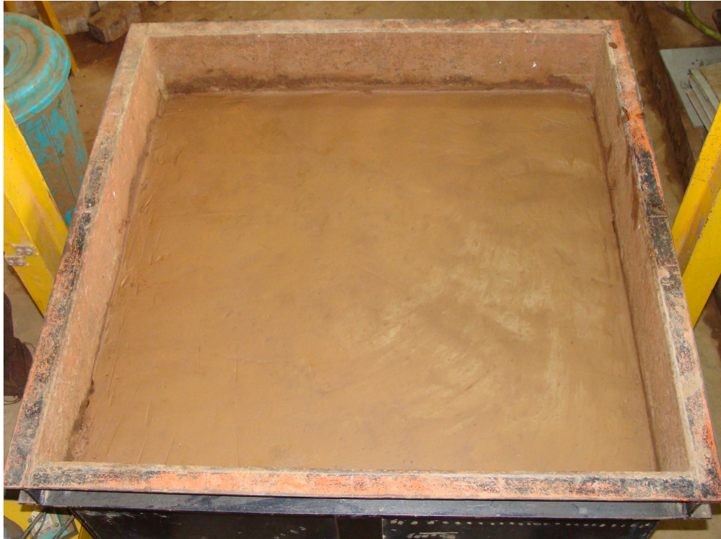
Fig. 3.38: Photograph of a typical clay bed in the test tank
