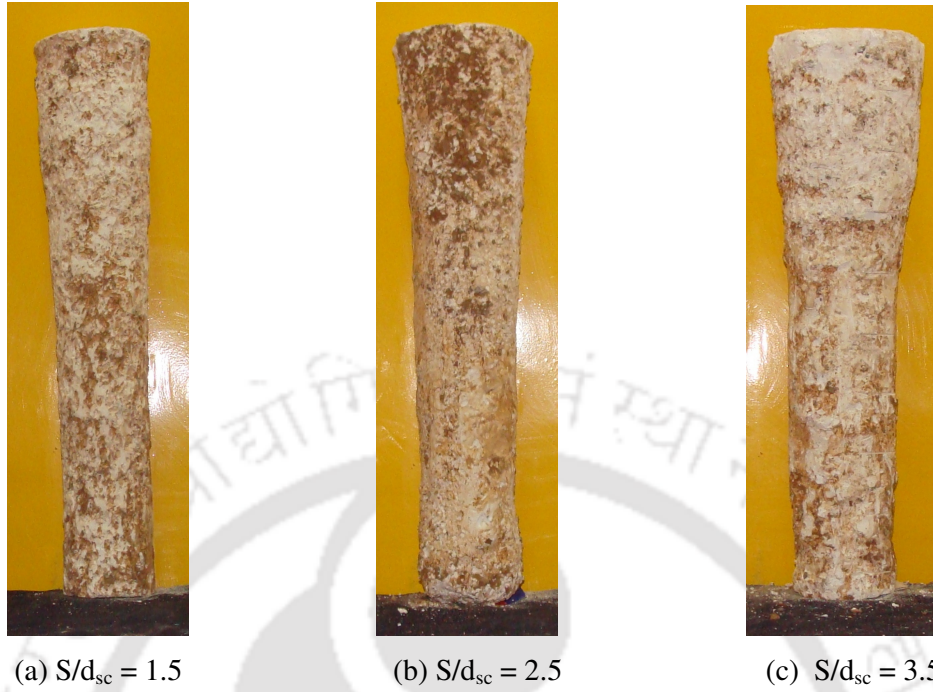
Fig. 6.61: Post-test deformed shape of central stone columns in composite foundation bed ( h/D = 0.9, L/d_{sc} = 5 ) – Test series 14
