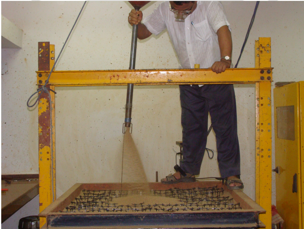
Fig.3.42: Photograph of sand raining for filling up geocell pockets
