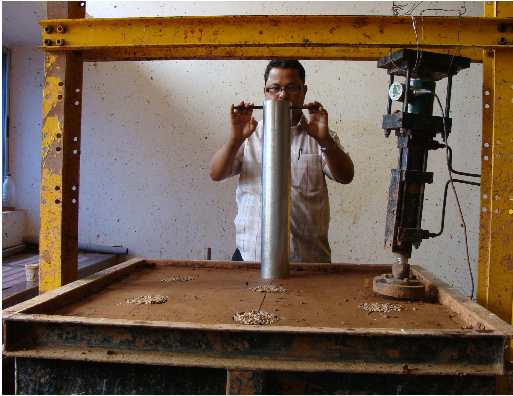
Fig.3.39: Photograph showing the construction of stone column
