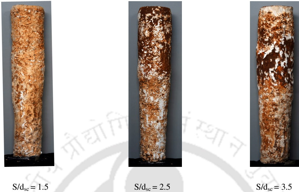
Fig.4.21: Deformed shape of central stone columns after test ( L/d_{sc} = 5 ) – Test series 3
