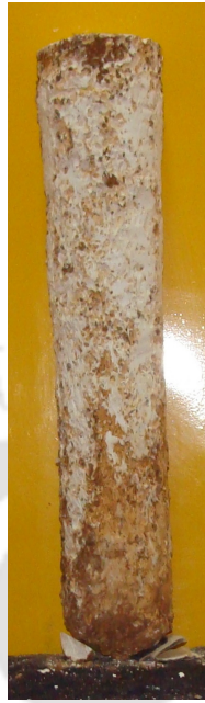
Fig.6.45: Post-test deformed shape of a typical central stone column in composite foundation bed ( L/d_{sc} = 5 , h/D = 1.6 , S/d_{sc} = 2.5 ) – Test series 12
