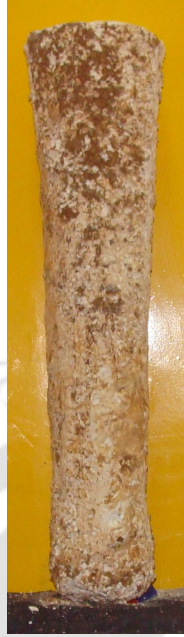
Fig.6.25: Post-test deformed shape of a typical central stone column in composite foundation bed ( L/d_{sc} = 5 , h/D = 0.9 , S/d_{sc} = 2.5 ) – Test series 10
