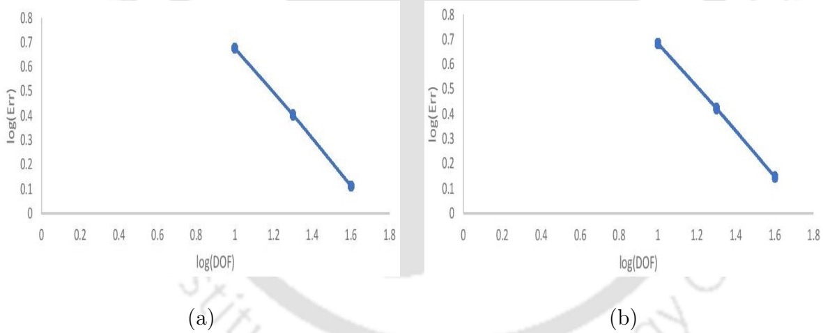
Figure 3.6: Energy error versus number of degrees of freedom: (a) \beta_1 = 1, \beta_2 = 10 and (b) \beta_1 = 1, \beta_2 = 100 . The quasi-optimal decay is observed by the line of slope -0.837 (left) and the line of slope -0.893 (right).
