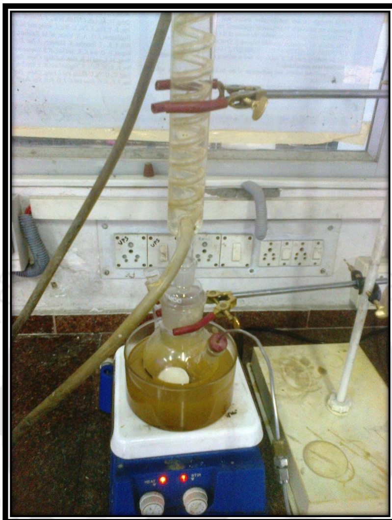
Figure 6.3 Experimental set-up for amine functionalization for OMS membrane
