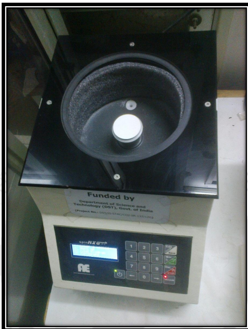
Figure 6.2 Spin coater Instrument for membrane coating
