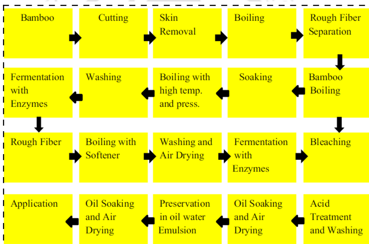
Fig. 1.8: Extraction of rough and fine bamboo fiber [42].
