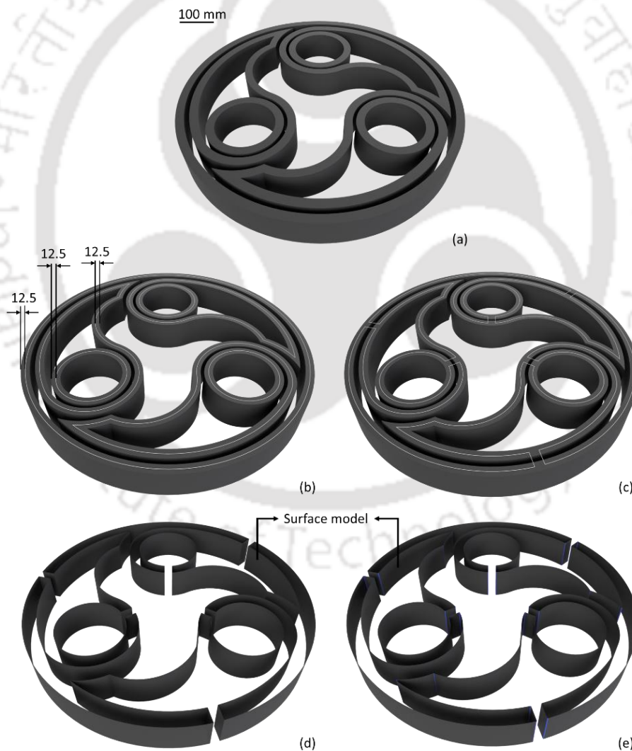
Figure 2.9 Stepwise development of 2.5D surface model for AMoC: (a) Orientation selection, (b) Surface offset for 25 mm bead width and 10 mm layer height, (c) ACAP toolpath generation, (d) Extrusion of the ACAP path to the full geometry height, and (e) Sharp junctions elimination
