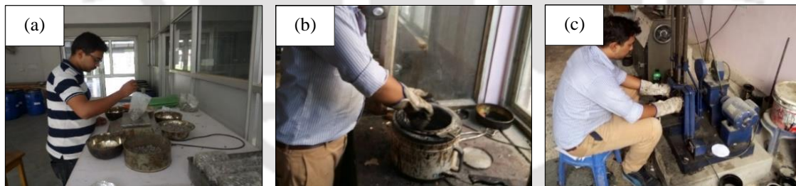
Figure 3.8: Preparation of OGAFc mixes: (a). Batching of aggregates, (b). Mixing of OGAFc samples, and (c). Compaction of OGAFc samples.
