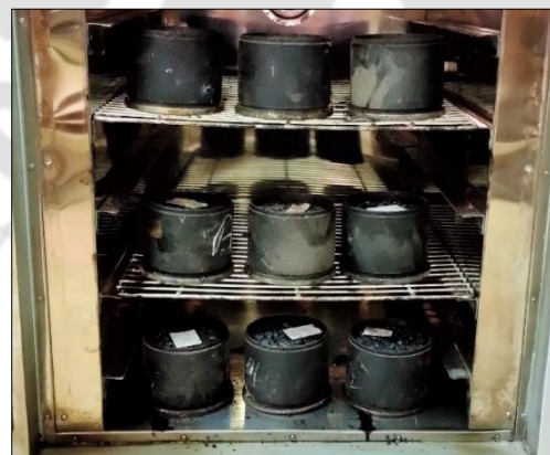
Figure 3.34: Simulation of long-term binder draindown by conditioning at 160°C.
