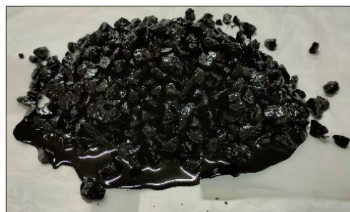
Figure 3.14: Binder draindown observed in OGAFc mixes.
