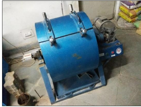
Figure 3.16: Los Angeles abrasion drum used for Cantabro abrasion loss test.
