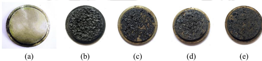
Figure 6.8: Photographs showing drained binder on base plate (4-inch diameter) after long-term draindown conditioning (8 hours at 160°C): (a) base plate before testing, (b) control PMB-OGAFc, (c) 100% slag PMB-OGAFc, (d) control CRMB-OGAFc, and (e) 100% slag CRMB-OGAFc.
