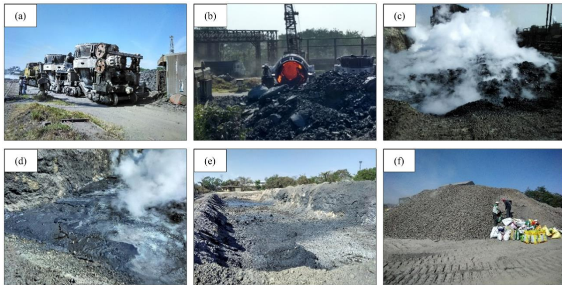
Figure 3.2: Processing and collection of BOF steel slag – (a) transfer of molten slag, (b) disposal of molten slag, (c) water spraying over molten slag, (d) water cooling process, (e) cooled steel slag, and (f) slag stockpiles.
