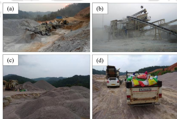
Figure 3.1: Processing and collection of natural stone aggregates– (a) aggregate crushers, (b). aggregate screening, (c). aggregate stockpiles, and (d). transportation of aggregates.
