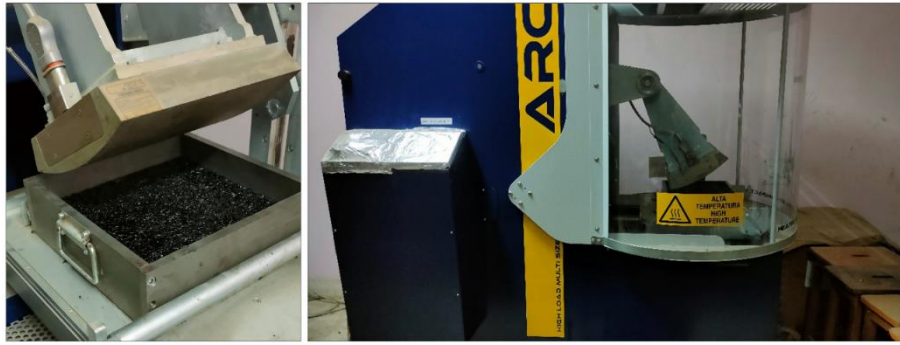
Figure 3.24: Roller compactor for preparation of square slab specimens.
