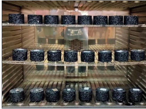
Figure 3.33: Simulation of long-term binder draindown by conditioning at 60°C.
