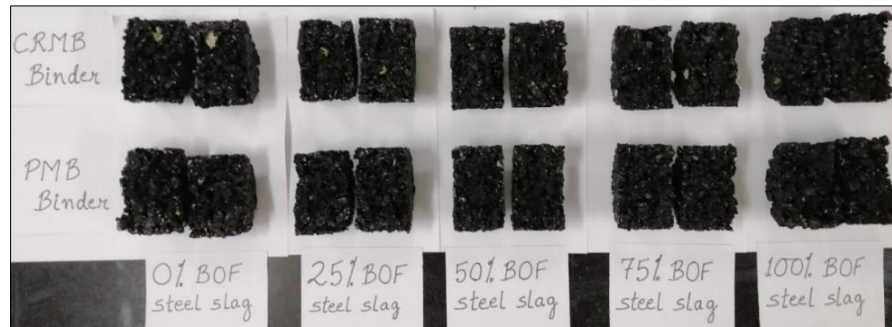
Figure 6.2: Fractured surfaces of specimens from indirect tensile strength tests (conditioned under acidic environment).
