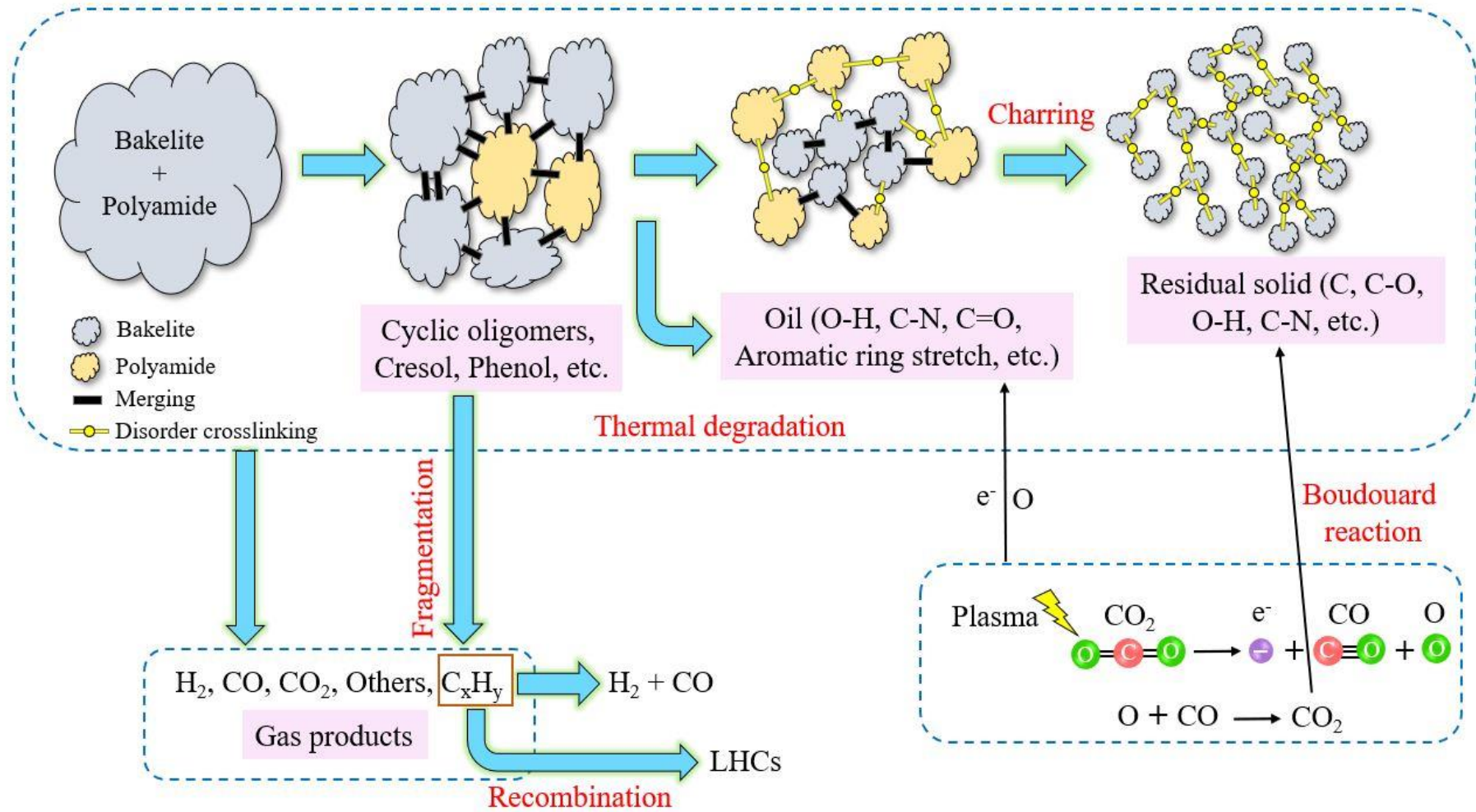
Fig. 6.11. Reaction mechanism of ESW in a plasma gasification process under CO 2 atmosphere.
