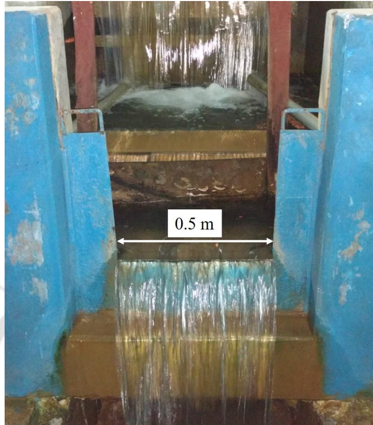
Figure 2.4 Rectangular notch for discharge measurement.
