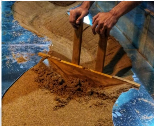
Figure 2.12 Preparation of the sinuous channel in the flume with wooden shaper and stencil.
