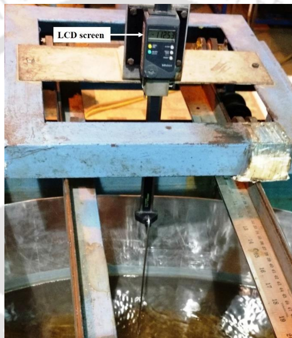
Figure 2.6 Digital point gauge.
