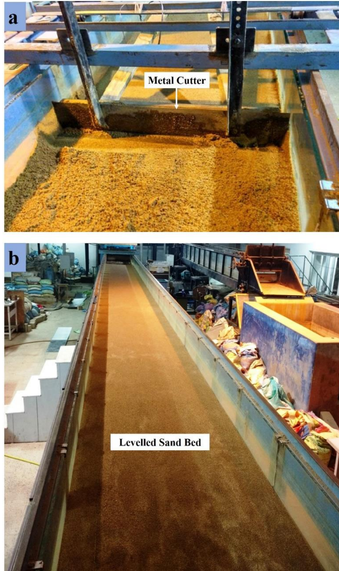
Figure 2.11 Levelled sand bed preparation with metal cutter.
