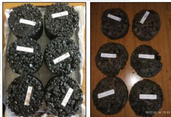
Figure 3.22: Comparison of the specimen before (left) and after (right) wet abrasion loss testing
