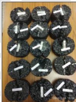
Figure 3.31: Sample failure along the central part of the vertical diameter
