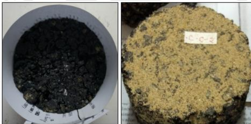
Figure 3.13: Clogging of OGFC sample
