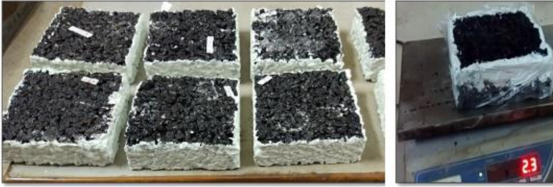
Figure 3.18: OGFC mix slab wetting protocol
