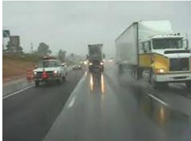
Figure 2.2: Glare in wet weather conditions (on left: OGFC layer, on right: dense graded layer) (Kandhal and Mallick, 1999)
