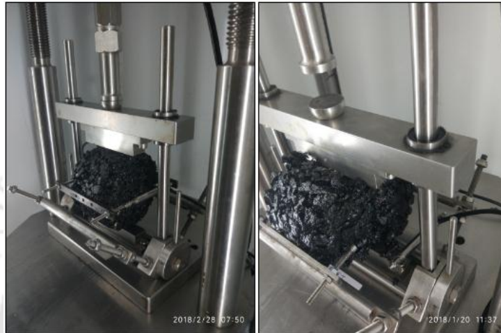
Figure 3.30: Test setup and failure of samples during ITFT test
