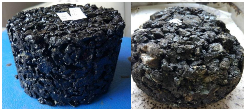
Figure 3.9: Comparison of the specimen before (left) and after (right) Cantabro testing
