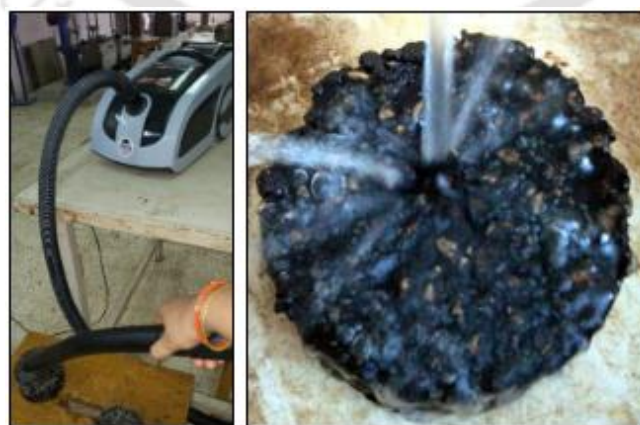
Figure 3.14: De-clogging of OGFC samples by (a) vacuum cleaner (b) Tap water
