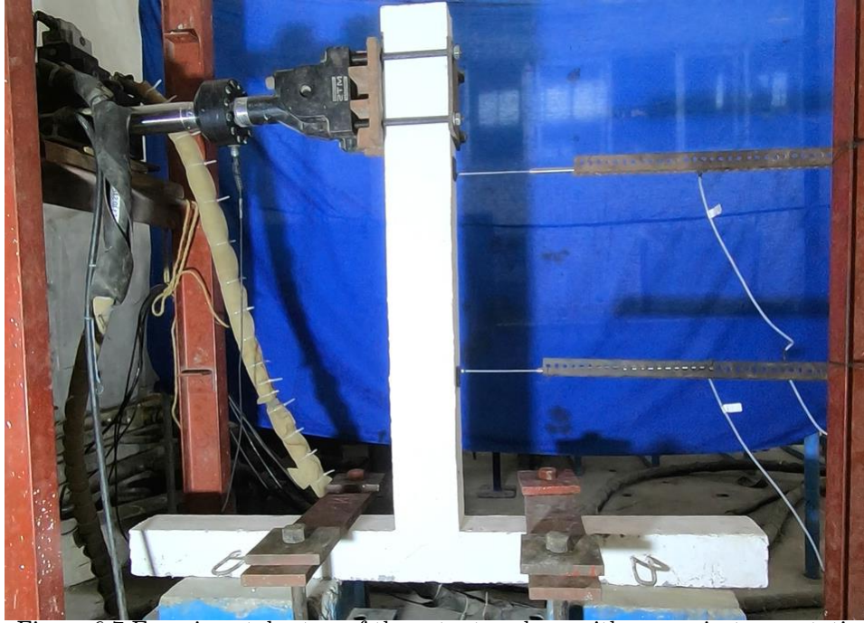
Figure 6.7 Experimental setup of the actuator along with sensor instrumentation
