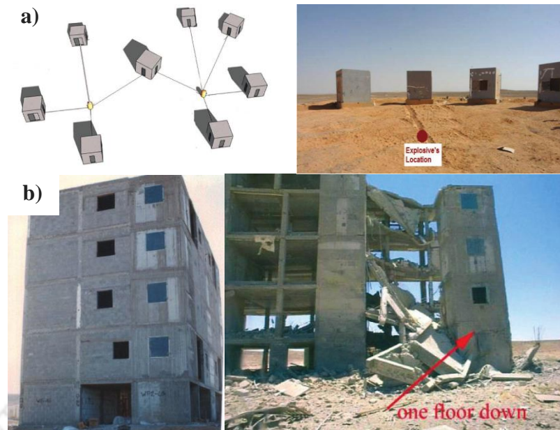
Figure 2.5 Representative schematic arrangement of cubicle specimens blast test arena and arenas of cubicles [before and after] (Yankelevsky et al. 2013)
