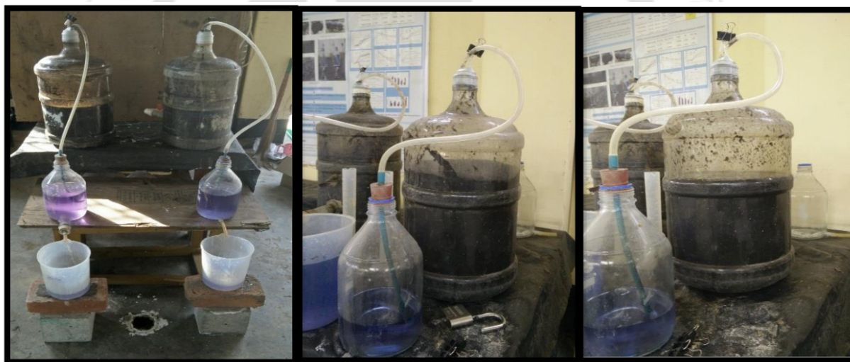
Fig. 3.6. Batch reactor setup with water displacement system
