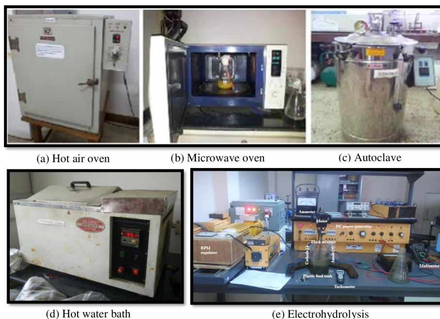
Fig. 3.4. Instrumentation used for the pretreatment study
