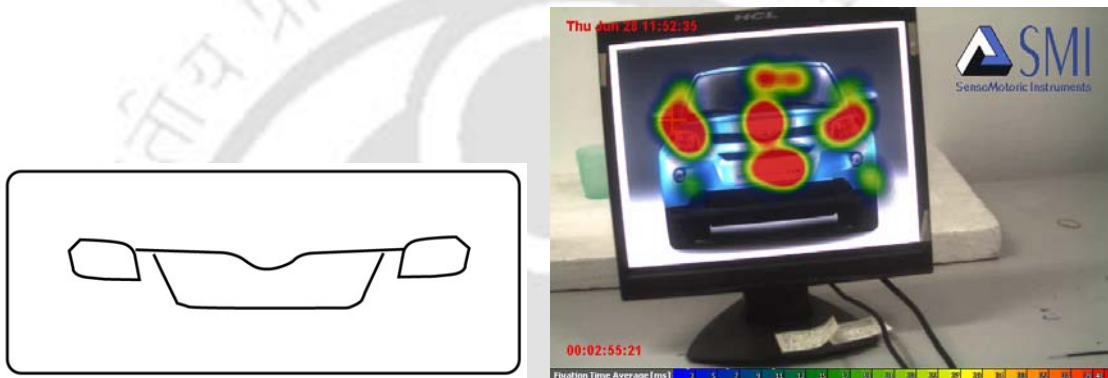
Figure 5.2a.41: Graphical key of H3 (Left), Eye tracking analysis of H3 (Right) Proportion analysis reveals that the, H3 is powerful in terms of both geometric and golden ratio. The visual hierarchy analysis shows, that the eye movement first moves to the location of grille “A” due to the existence of the golden ratio area and also due to the presence of contrast of colors. The eye wanders from grille and logo “A” to lights “B” because of the color. It may hence be concluded that the icon grille “A” is a very attractive search icon within the peripheral field of vision. The result of machine eye tracking analysis shows the eye jump from grille and logo “A” to lights “B”. In terms of sequences it is 100% same with the result of self assessment eye movement analysis and in terms of importance of elements both result shows same locations which is visible in the above figure.
