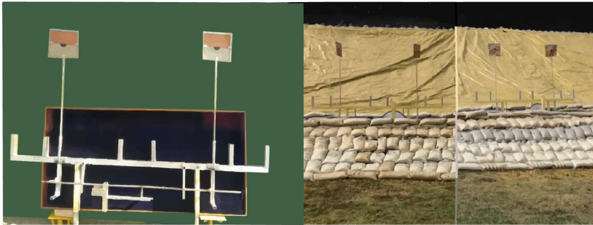
Figure 3.5 : Specially Designed Target Flip Mechanism of Mod 3
