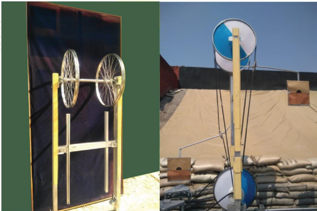
Figure 3.4 : Photo of \Pi -structure with target-guide mechanism (LHS), along with Photo of Complete Mod 2 Assembly (RHS)
