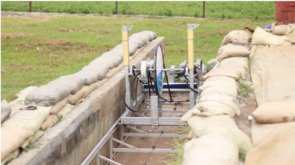
Figure 3.2 : Chassis with Custom Designed Superstructure
