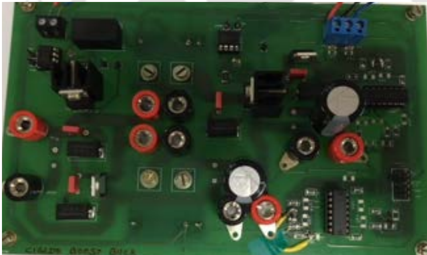
Figure A.9: Prototype of CI-SIDO boost and buck converter
