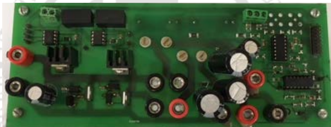
Figure A.3: Prototype of CI-SIDO buck converter
