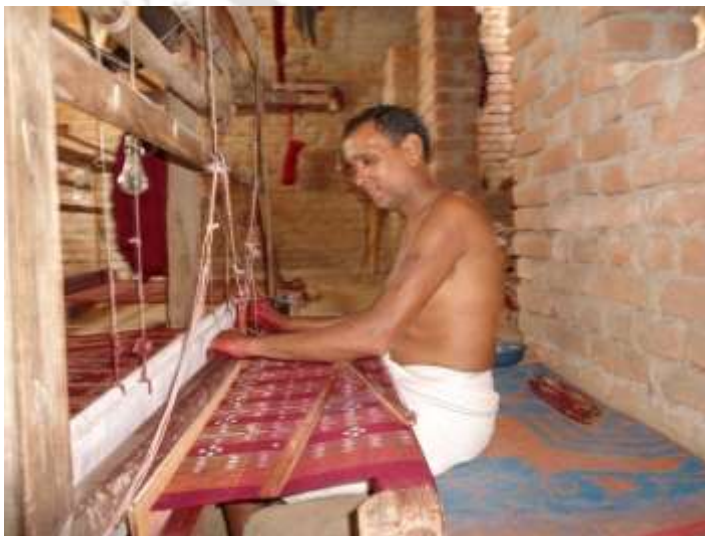
Fig. 2.10 Weaver weaving Ikat Sari on the Handloom
