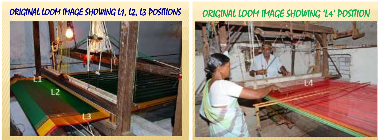
Fig. 3.6 Original loom image signifies the positions L 1 , L 2 , L 3 and L 4 for measuring the illumination values.
