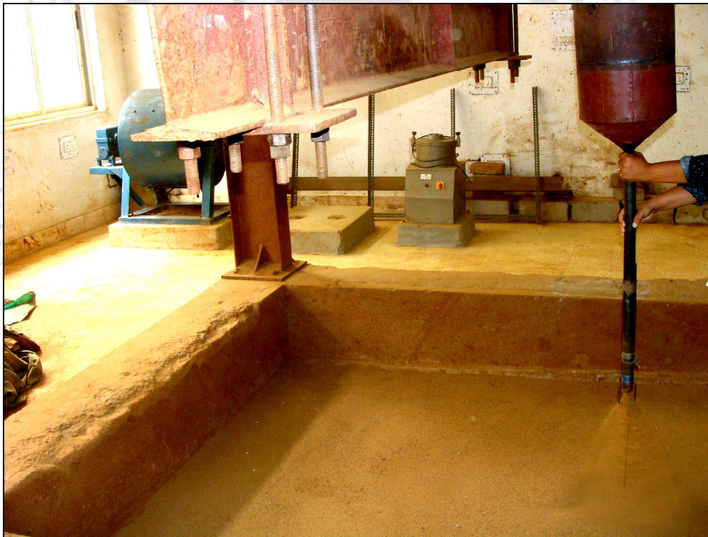
Photo 3.5 Sand raining in progress
