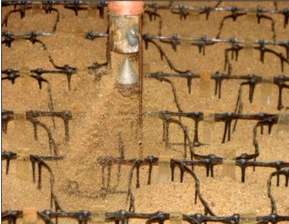
Photo 3.6 Sand raining in progress
