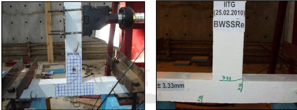
Fig. 4.13 Test set up for BWSS specimens and typical appearance of initial cracks under loading type-1
