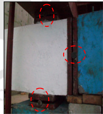
Fig. 2.10 Roller support at column end
