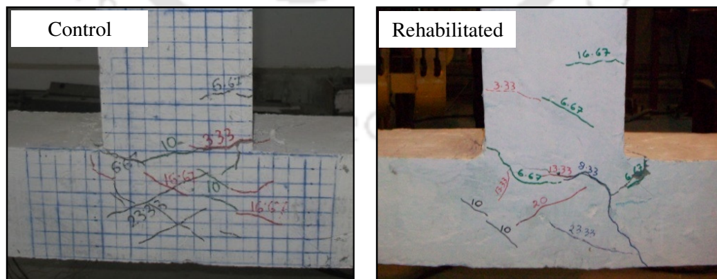
Fig. 4.7 Appearance of cracks for BWSM specimens under loading type-1 corresponding to peak load
