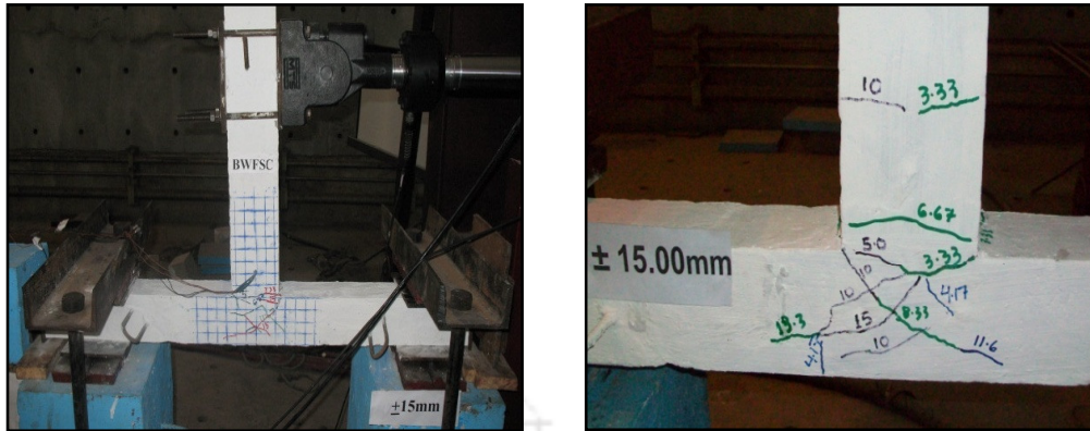
Fig. 3.12 Test set up for BWFS specimens and cracking pattern under loading type-1
