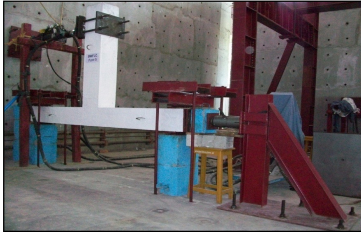
Fig. 2.11 Test arrangement for large and medium specimens
