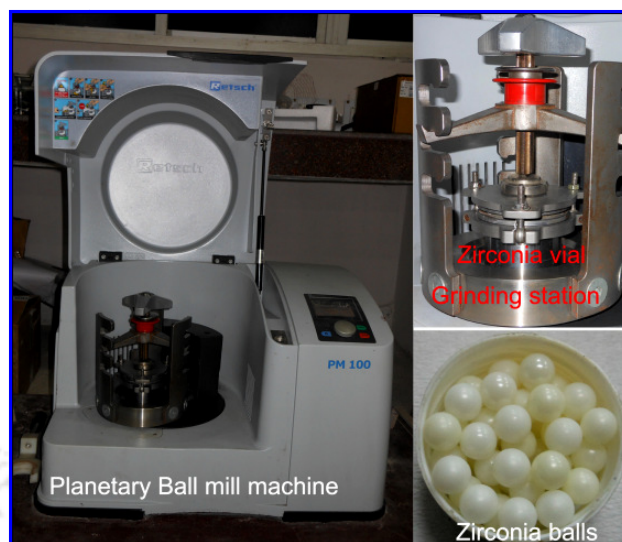
Fig. 2.3. Photographs of the planetary ball-mill machine (Retsch, PM 100), grinding station and Zirconia balls.
