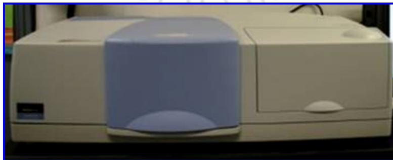
Fig. 2.9. Photograph of the Diffuse Reflectance Spectrometer (Perkin Elmer, LAMBDA 750).
