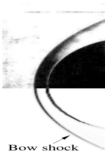
Figure 4.15: Comparison of numerical Schlieren (below) and experimental Schlieren (top) [117] for hypersonic flow over sphere
