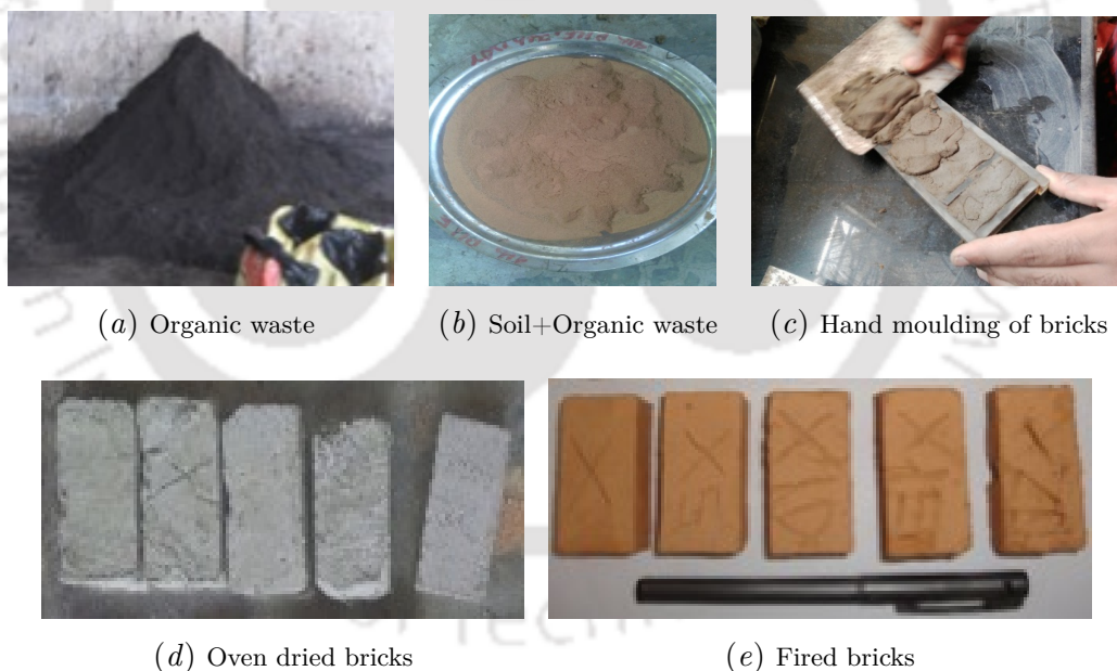
Fig. 3.4. Brick manufacturing process
