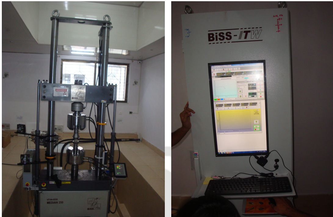
Fig. 3.5. Universal testing machine (UTM, BISS, Median-250)
