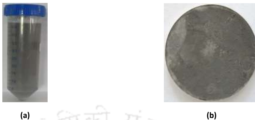
Figure 3.1: Photographs of (a) spent ELP solution and (b) Pd/PSS composite membrane obtained with 0.02 M SOEP Pd bath and 30 min. plating time.
